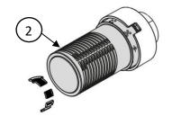
2. Turn the operating device (2) counterclockwise until you reach the position "completely open" identified by the symbol
