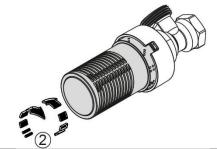
4. Select the desired position by turning the device
